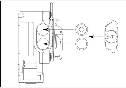
Figure 12: Installing the Alkaline Batteries
