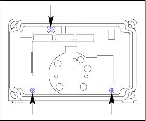
Figure 23: Reinstalling Battery Board Screws
