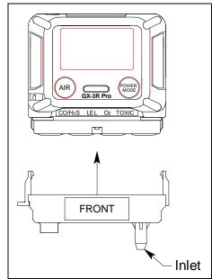
Figure 10: Calibration Cup Installation
