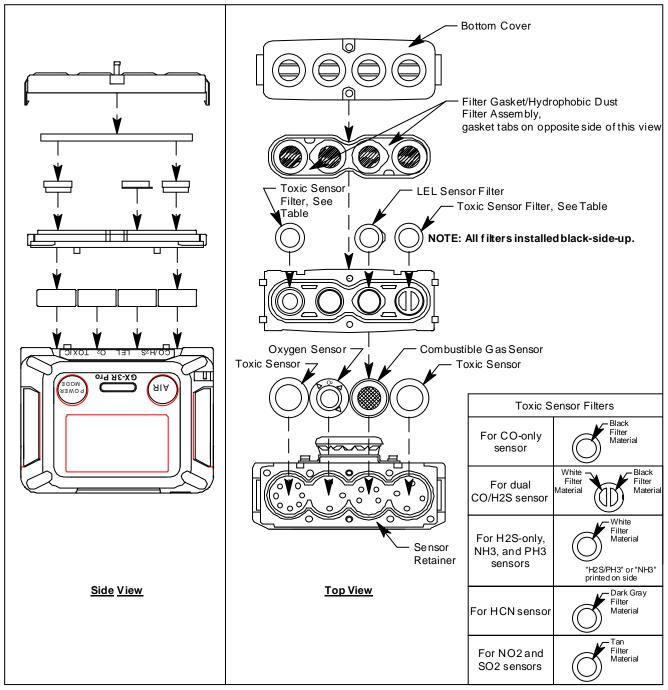
Figure 18: Replacing a Sensor
