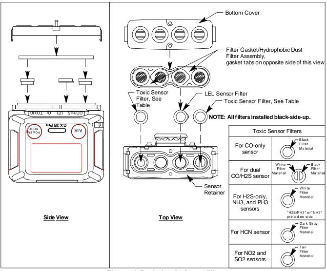
Figure 16: Replacing the Sensor Filters
