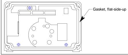
Figure 24: Reinstalling Battery Board Screws
