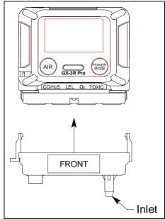
Figure 9: Calibration Cup Installation
