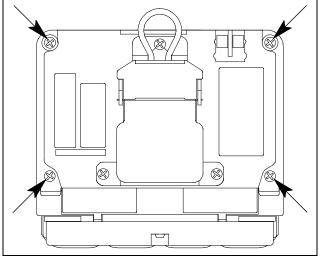
Figure 25: Reinstalling Case Screws
