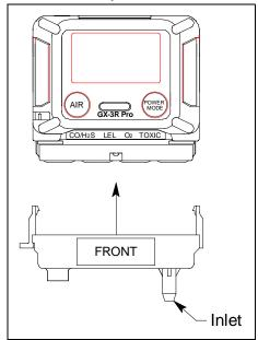
Figure 7: Calibration Cup Installation
