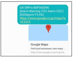
Figure 27: Text Alert for CO<sub>2</sub> Warning and Alarm
