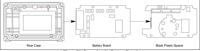
Figure 21: Removing the Battery Board
