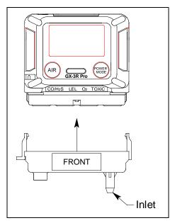
Figure 28: Calibration Cup Installation
