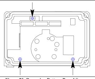
Figure 20: Removing Battery Board Screws
