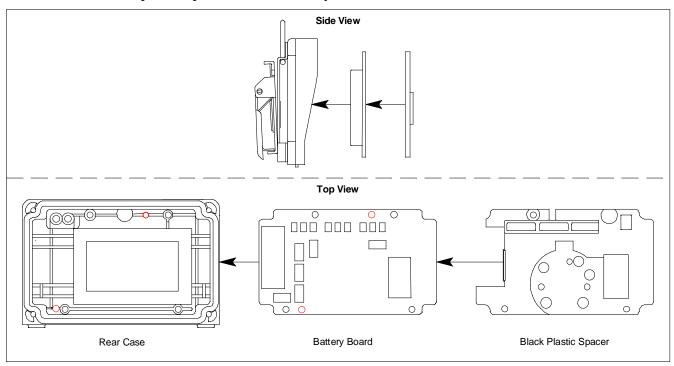
Figure 22: Reinstalling the Battery Board
