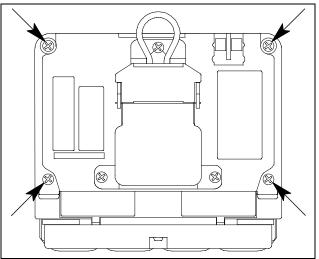
Figure 19: Removing Case Screws
