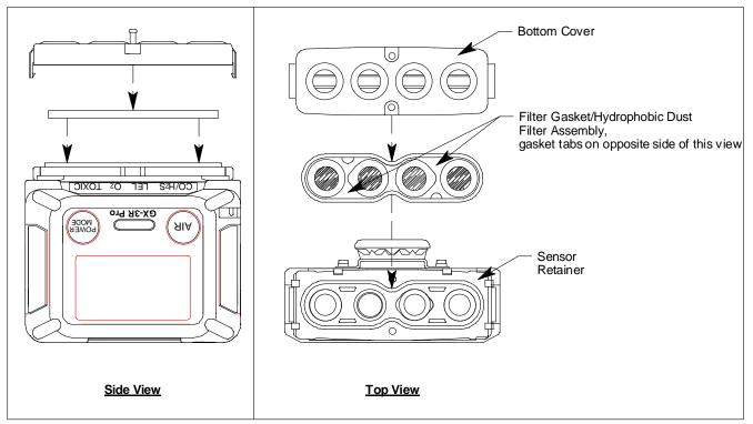
Figure 17: Replacing the Hydrophobic Dust Filter
