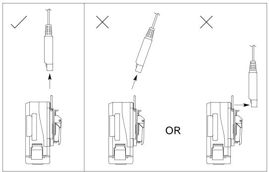
Figure 14: Removing the Charging Cable
