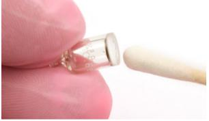
Figure 9: Polishing the Electrode Lamp Window
