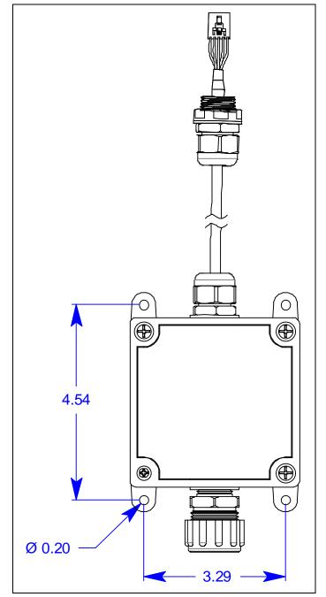
Figure 5: Remote-Mounted Kit's Detector Junction Box Dimensions
