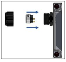
21. Screw the sensor housing cap back onto the sensor housing base, ensuring that the sensor housing cap is only tightened hand tight.
