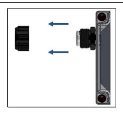
3. Gently unplug the sensor element from the sensor housing board.
