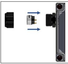
15. Screw the sensor housing cap back onto the sensor housing base, ensuring that the sensor housing cap is only tightened hand tight.
