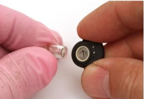
Figure 10: Reinstalling the Electrode Lamp
