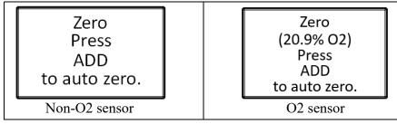
2. Press the ADD button to begin the zero process and advance to the clean air confirmation screen.
