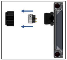
4. Plug the new sensor element into the sensor housing board. Ensure that the pins on the sensing element align with the sockets on the sensor housing board.
