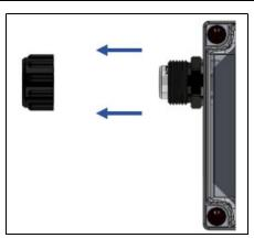
3. Gently unplug the sensor element from the sensor housing board.
