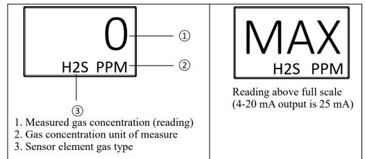
The gas reading is sent back to the controller in 1-minute intervals when the reading is below the background setting (page 28). When the reading surpasses the background setting, the reading is sent back to the controller in 5-second intervals.
