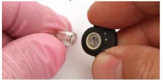
Figure 12: Reinstalling the Electrode Lamp
