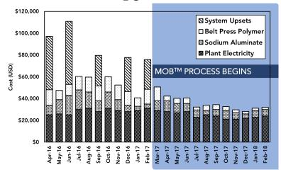
**Figure 7. Monthly cost breakdown** of the Moorefield WWTP since April 2016. The MOB<sup>™</sup> Process has decreased the total monthly usage as well as individual usage in electricity, sodium aluminate, and belt press polymer. More importantly, the MOB<sup>™</sup> process has eliminated system upsets since the March 2017 installation.
