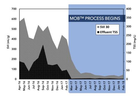
**Figure 10. 30-min Sludge Volume Index (SVI30) and Effluent TSS** decreased significantly from an average of 460 mL/g and 90 mg/L to an average of 60 mL/g and 4 mg/L, respectively since March 2017.
