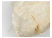
Figure 5. Kenaf particles have a highly textured surface to support biofilm growth. 2
