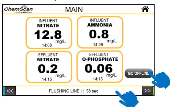
To exit the on-line mode, press the GO OFFLINE Button **OR** in **any** screen press the Analysis Message Bar at the bottom.
