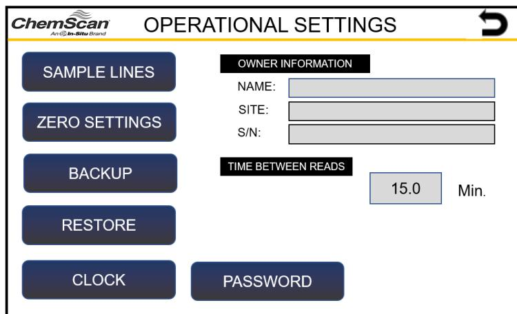
The Operational Settings screen for ChemScan. It features a sidebar with buttons for SAMPLE LINES, ZERO SETTINGS, BACKUP, RESTORE, CLOCK, and PASSWORD. The main area has sections for OWNER INFORMATION (NAME, SITE, S/N) and TIME BETWEEN READS (set to 15.0 Min.).
