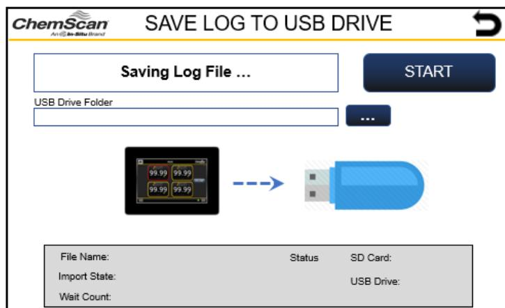
The analyzer's Concentration Data Log can be extracted to an USB drive by pressing the START button.
