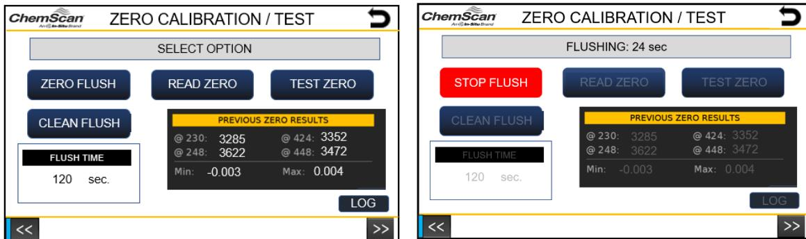
Press the ZERO FLUSH button to begin flushing the deionized water. Allow the water to flush for 2 minutes and press STOP FLUSH to stop flushing. Allow the water to settle in the flowcell for 10 – 15 seconds.
