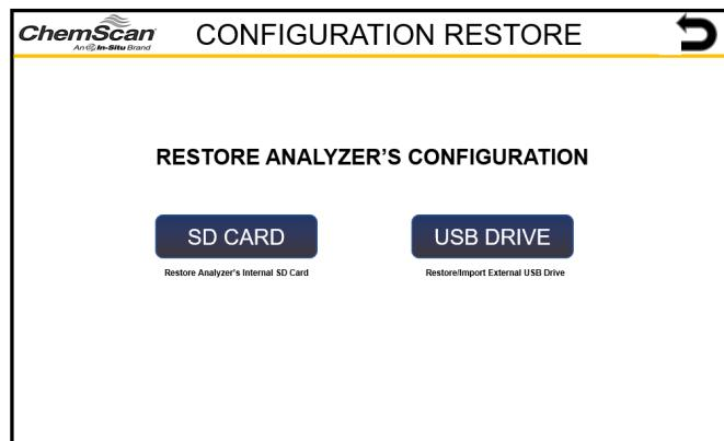
**SD CARD** button will restore the configuration stored on the internal SD card.
