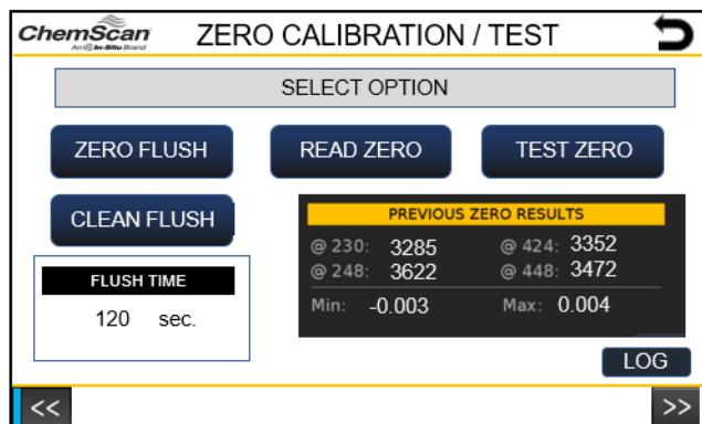
Press the ZERO FLUSH button to begin flushing the deionized water. Allow the water to flush for 15 – 20 seconds and press STOP FLUSH to stop flushing. Allow the water to settle in the flowcell for 10 – 15 seconds.
