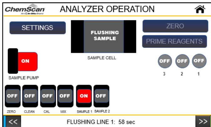
While in On-Line Mode the Analyzer Operation Screen will display status of the components during the analysis cycle. The Analyzer's operational SETTINGS Screen can be displayed but the edit function is disabled. The ZERO and PRIME REAGENTS buttons are disabled. Exit the On-line Mode to enable the ZERO and PRIME REAGENTS buttons and allow editing of the operational SETTINGS.
