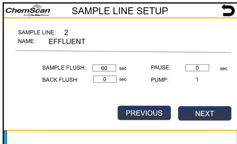
The Sample Line Setup screen for ChemScan. It shows a current sample line setup for Sample Line 2, named EFFLUENT. It includes fields for SAMPLE FLUSH (60 sec), PAUSE (0 sec), BACK FLUSH (0 sec), and PUMP (1). Navigation buttons PREVIOUS and NEXT are at the bottom.
