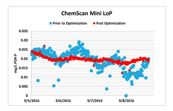
The ChemScan mini LoP analyzer's simplified design makes it easy to operate, maintain and adjust. Through configuration changes, the analyzer performance has been optimized to reduce the reading variability significantly.
